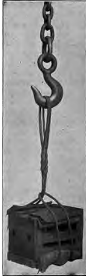
FIG. 36.—Single cable sling lifting load (wrong way).
